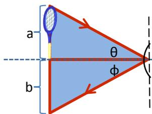
Hint: you don't need a protractor to accurately draw the ray that reflects from the vertex of the mirror. Simply measure the height of the object, draw a dot the same distance below the principal axis, and then draw in the reflected ray from the vertex to the dot. In the diagram on the left, you can see that if the two lengths "a" and "b" are the same, then the two angles  $\theta$  and  $\phi$  are the same, too.
