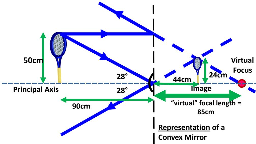
$$\text{magnification} = \frac{\text{height of image}}{\text{height of object}} = \frac{24\text{cm}}{50\text{cm}} = 0.48$$
