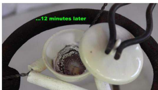
This strip of magnesium has a mass of 0.184grams, the crucible and lid have a mass of 23.767 grams and the combined total is 23.951 grams. If we heat the magnesium in the crucible, it eventually starts to burn. By placing the lid on the crucible, we can slow the burning process and limit the amount of smoke that escapes. The magnesium metal eventually turns into a whitish powder, which is called magnesium oxide, because the magnesium atoms and oxygen atoms from the air have joined together.
