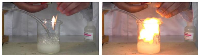
As the gas is produced, it passes through the tube into the soapy water and it's trapped inside the tiny bubbles which form. This gas is not like oxygen which supports fire, it's actually flammable. In 1783, it was named "hydrogen".
