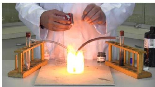
To show you the water forming, we can also collect hydrogen gas in a dry upside down test tube and then ignite it. It's very hard to see, but the inside of the test tube is now a little misty because some of the water that was produced in the reaction has condensed on the glass.
