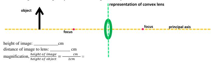
15. Skill-Building Exercise: A 2cm-tall object stands 9cm from a convex lens of focal length 3cm. Determine the height of the image, its position, and the magnification produced.
