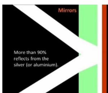
A mirror is made of a **layer of glass** onto which a reflective **layer of silver or aluminium** is applied with the help of certain chemicals. Over the top of
