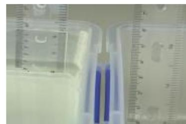
From above, there's not much difference, because the light coming from the bottom of the ruler travels almost straight up and doesn't refract much; as your angle gets lower, the distortion increases, because the light refracts more.
