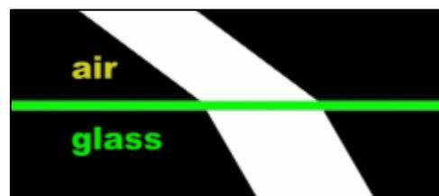
When a light beam goes from glass to air, the side of the light beam that hits the air first will speed up first so the light beam bends the other way.
