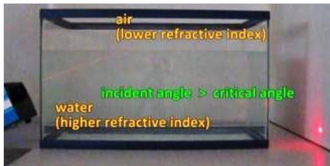
Here a laser beam is shining upwards into a fish tank with some dirty water in it. The dirt scatters some of the laser light which allows us to see its path. Since water has a higher refractive index than air and the light is hitting the undersurface of the water at an angle greater than the critical angle for water, which is 49 degrees, it totally internally reflects.
