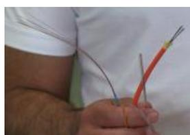
Finally, probably the most important use of total internal reflection in everyday life is in optical fibres. Inside this optical fibre cable are a number of optical fibres. Optical fibres are extremely thin, flexible glass fibres which are used to carry data in the form of light beams from one place to another in communications networks.
