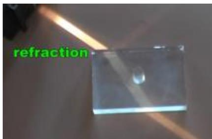
Here, for example, the light beam traveling in the air hits a glass block at an angle and then changes direction, or bends, when it enters the glass block. The light beam has refracted. When the light beam then hits the other side of the glass block it passes from the glass block to the air and so it changes direction again. The light beam has refracted again.
