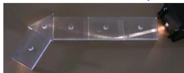
I can demonstrate what happens in an optical fibre by shining light into a row of perspex blocks. The light totally internally reflects when it hits the inside surface of the perspex, because it's hitting at an angle greater than the critical angle. I can simulate a bend in the fibre by adding a triangular block.
