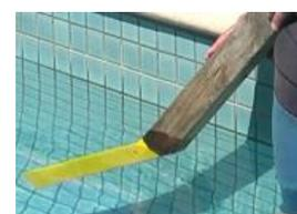
placed in water. Here, the bottom of the timber is actually about 40cm below the surface of the water, but it appears to be only about 20cm below.
