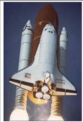
The space shuttle at launch has a mass of about 2 million kg and consists of 4 main parts.
